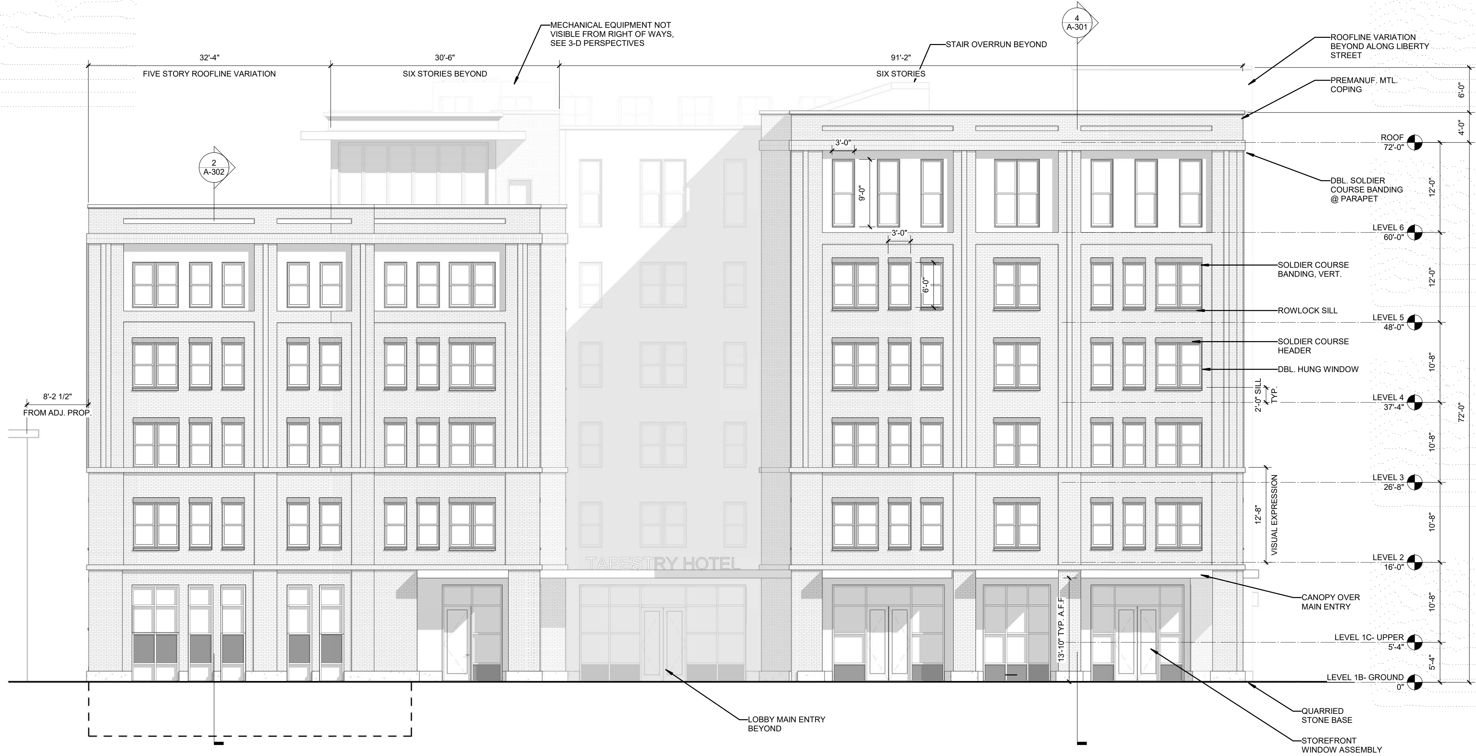
A1 ELEVATION- EXTERIOR- EAST 1/8" = 1'-0"
